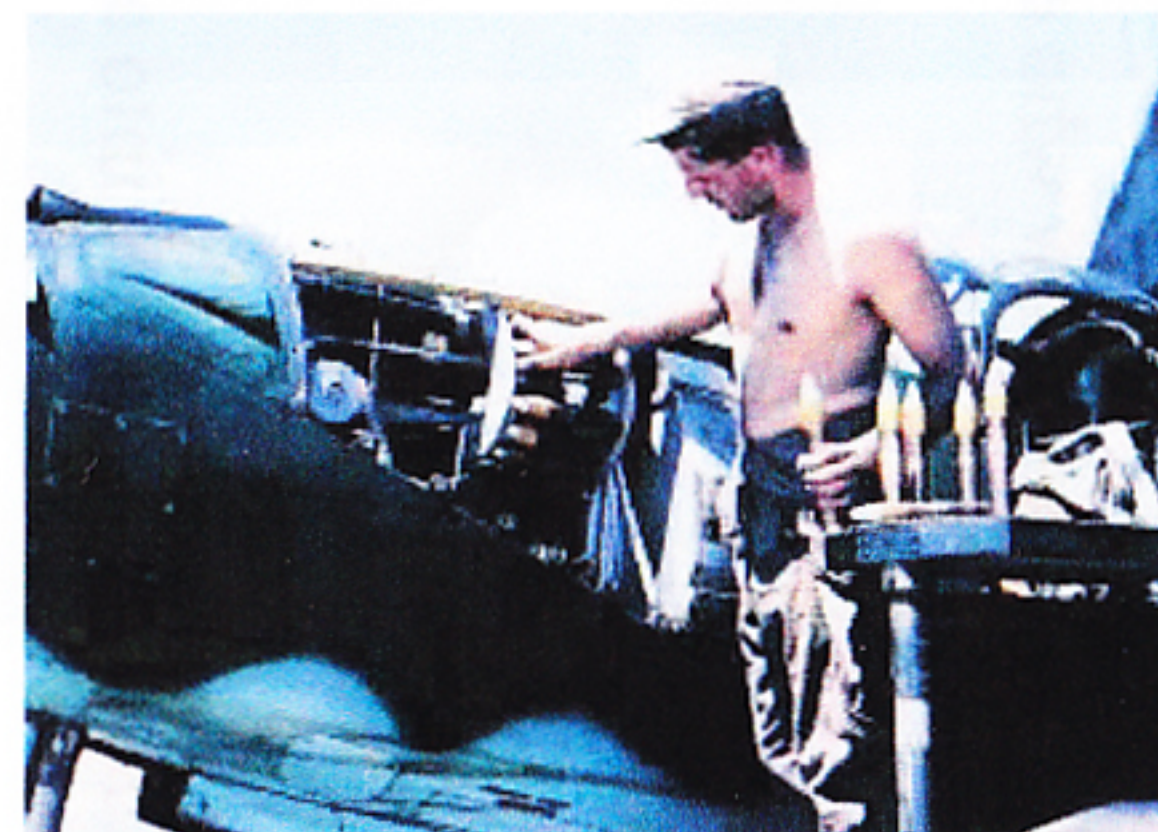
An armorer loads shells into the ammo magazine for the 37mm cannon that's located in the P-39's nose. (Photo courtesy of Stan Piet.)
