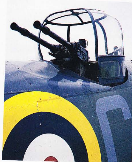
Initially, the Bristol Blenheim had a Bristol Type B.1. powered turret that was armed with a single Lewis machine gun. This turret armament was later changed to incorporate two Browning .303-caliber machine guns.
