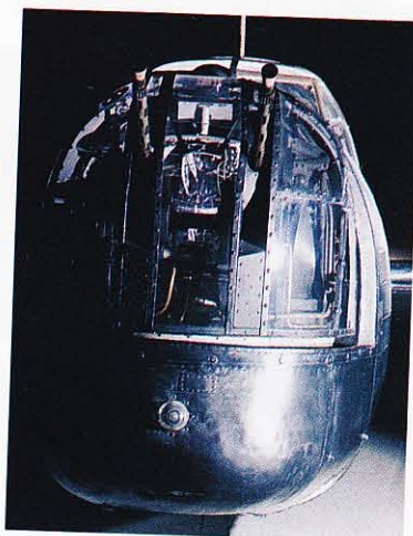
The Frazer-Nash nose turret of a Vickers Wellington.
