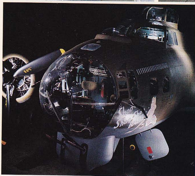
attacks, the B-17G model was equipped with a Bendix remote-control turret that was operated by the bombardier.
