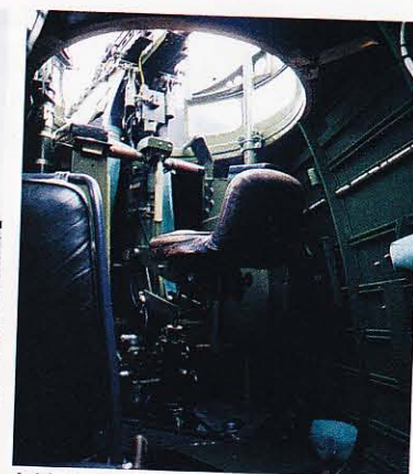
Initially, the Bristol Blenheim had a Bristol Type B.1. powered turret that was armed with a single Lewis machine gun. This turret armament was later changed to incorporate two Browning .303-caliber machine guns.
